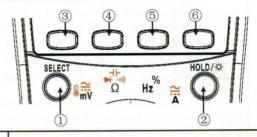
Selects alternate measurement modes on a rotary switch setting, including:
